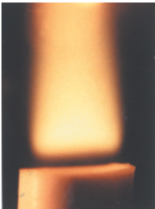
Figure 5-7. Flame photograph of TAGN burning at 0.2 MPa showing that the luminous flame front stands some distance above the burning surface.
