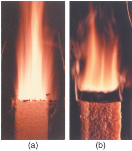
Figure 7-17. Flame photographs of AP composite propellant (a) and RDX composite propellant (b) showing that the luminous flame front of RDX composite propellant is distended from the burning surface:
